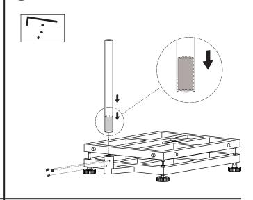
Remove Load Cell protection bolt and nut.
